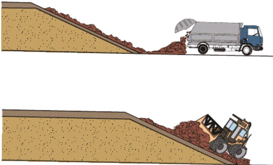
Figure 7: Illustration of the toe method of sludge co-disposal on landfill
