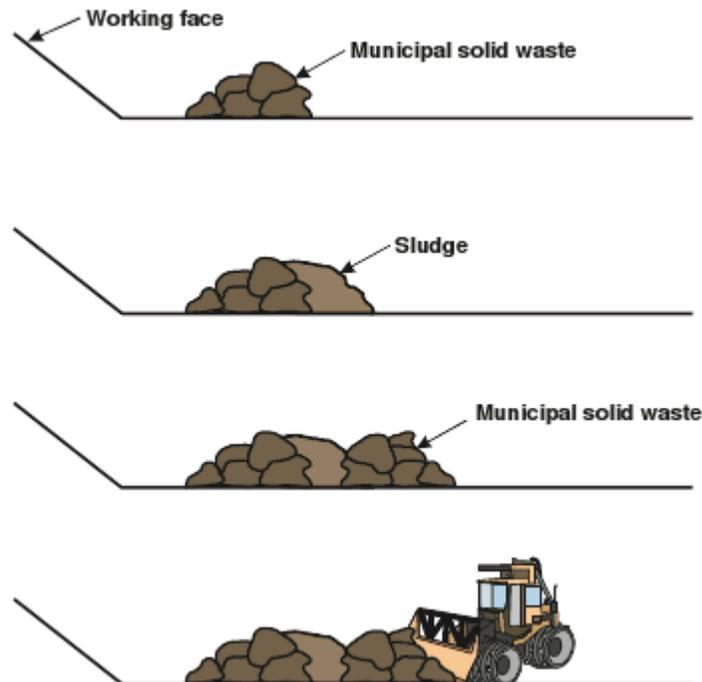
Figure 9: Proposed alternative method for sludge co-disposal on landfill
