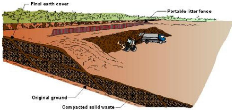
Figure 6: Illustration of the area method of sludge co-disposal on landfill
