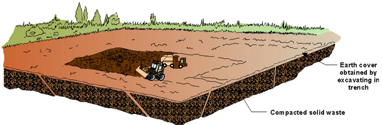
Figure 8: Illustration of the trench method of sludge co-disposal on landfill
