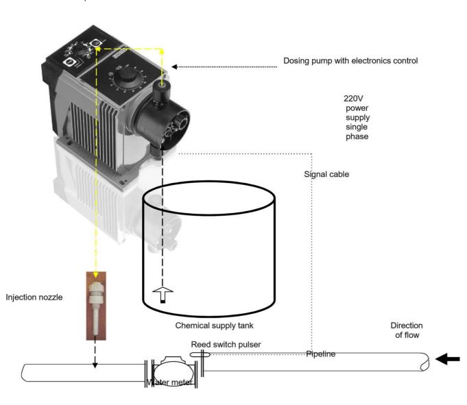
Dosing proportionate to flow shall be done with displacement pulse dosing pump with electronic control, interlinked with flow meter, read switch pulses.
