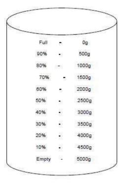
Tank level markings Mass of Calcium Hypochlorite to be added when filling with water Dosing proportionate to flow shall be done with displacement pulse dosing pump with electronic control, interlinked with flow meter, read switch pulses.
