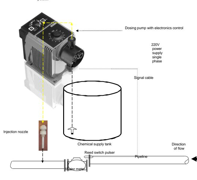
Dosing proportionate to flow shall be done with displacement pulse dosing pump with electronic control, interlinked with flow meter, read switch pulses.
