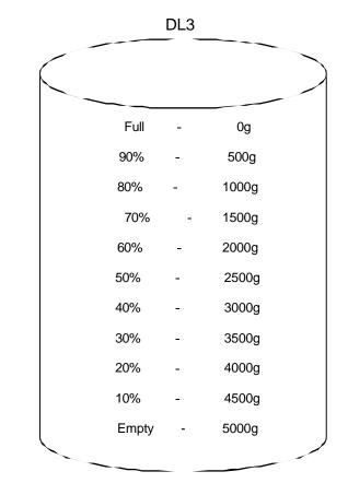
Tank level markings Mass of Calcium Hypochlorite to be added when filling with water
