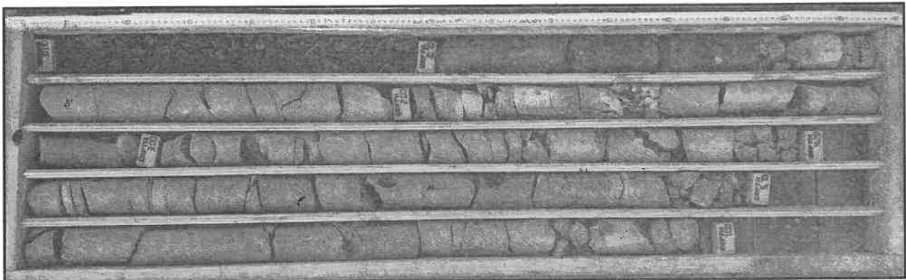
Plate 10: Soil and rock samples retrieved during the drilling of borehole BH3.
