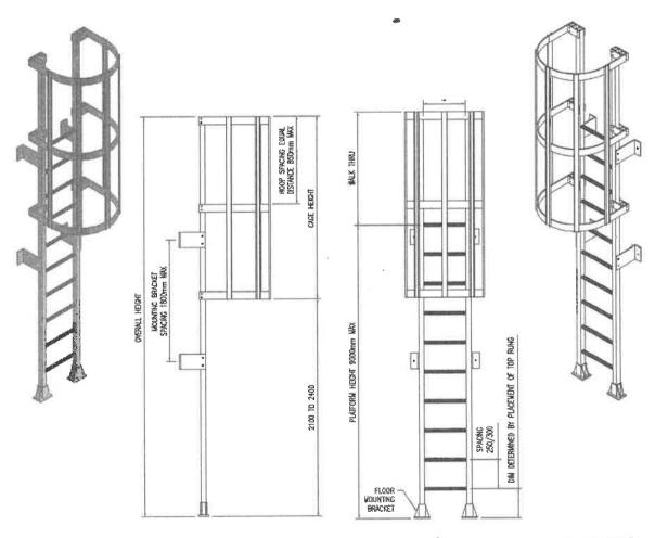
GALVANISED STEEL CAT LADDER INCLUSIVE OF SAFETY CAGE, FITTED TO BRICKWORK ALL AS PER GRATING WORLD OR SIMILAR APPROVED, TO FIT A HEIGHT OF 3,6M FLOOR TO FLOOR.
