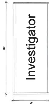
46 of 150 X 130 X 15mm anodized aluminium name plate with 15mm high suspended upper case. "Trace Balls Concealed" font lettering. 30 character per plate. Colour as per door number signage schedule. Plate fixed to door with double sided tape.
