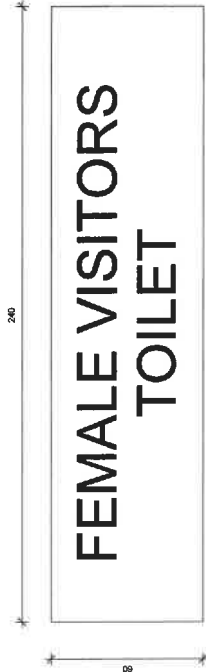
46 of 150 X 240 X 15mm anodized aluminium name plate with 15mm high suspended upper case. "Trace Balls Concealed" font lettering. 30 character per plate. Colour as per door number signage schedule. Plate fixed to door with double sided tape.
