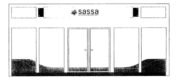
The shopfront illustrated is just an example of a typical corporate identity application and serves as a guideline. The Aluminium frame work of new shopfronts to be powder coated to match C3-7. If shop fronts are existing, it may remain in the natural aluminium or other colour. The fascia must however be in the corporate colours as indicated above with decals of the logo and our secondary curve graphic as indicated on the glass.
