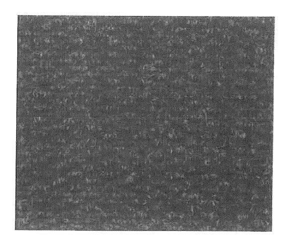
All SASSA offices must be carpeted with  $600 \times 600 \times 6.6$  mm Bilgotex Red Oxide Point 920 tiles. The colour of the carpet tiles has been chosen to obscure any dirt while at the same time being hardworking and durable. The carpet tiles are to be used in high volume areas, for example, receptions.
