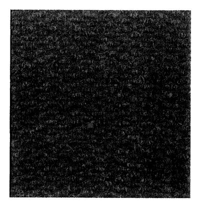
All offices to be carpeted with  $500 \times 500 \times 6.5 \text{rmm}$  Belgotex Red Oxide Berber Point 920 tiles. The colour of the carpet tiles has been chosen to obscure any dirt that may collect, while at the same time being very hard-working and durable. They are to be utilised in high volume area, especially reception areas.
