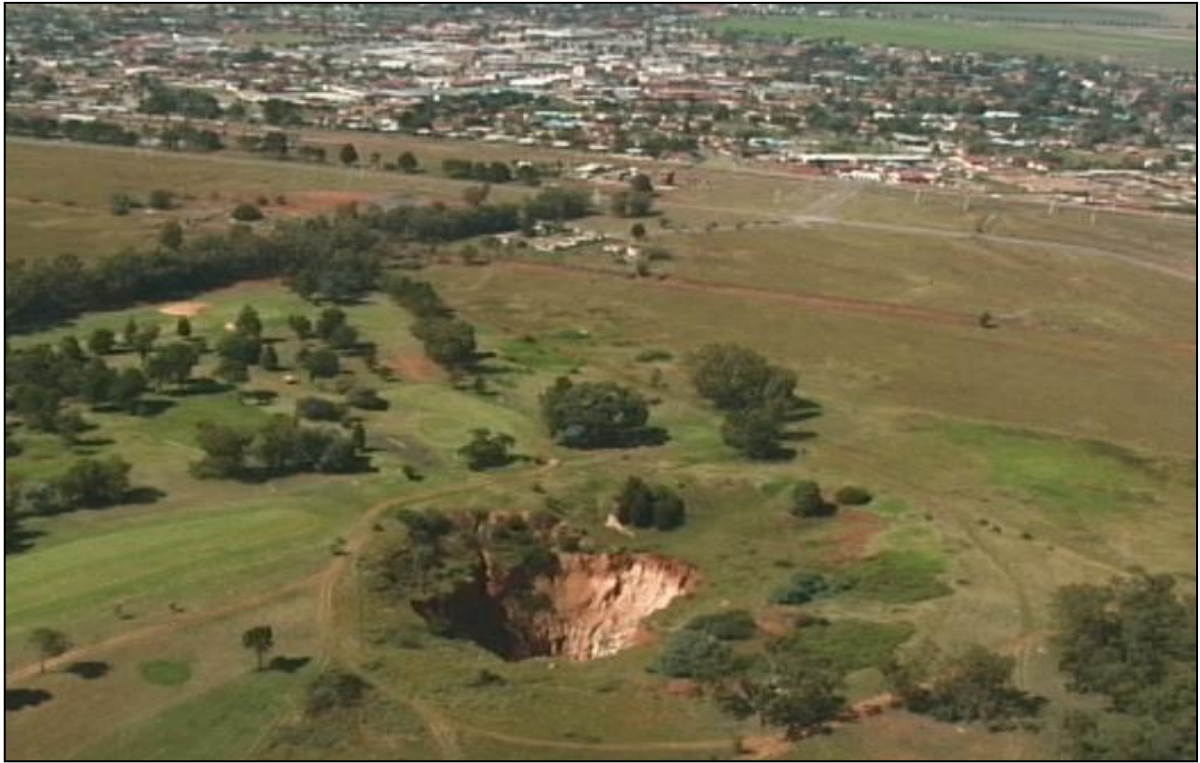
PLATE 7: Large sinkhole as result of dewatering
