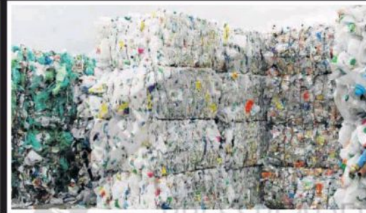
PLASTIC ROAD: Plastic is collected from rubbish dumps, packaged into bales and then melted down with bitumen to make a road
